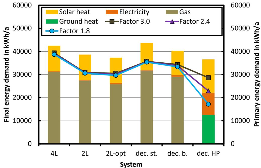
Fig. 8: Comparison of the final and primary energy demand of different systems
