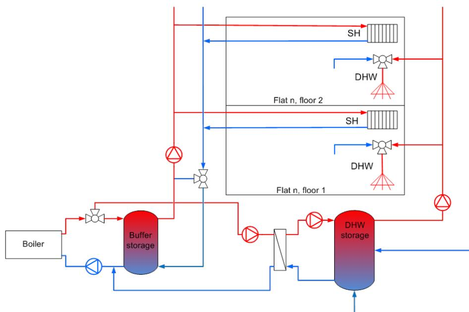
Fig. 1: Four-line pipe network with central heat generation
