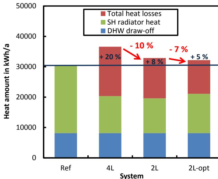
**Fig. 3: Impact of distribution pipe network optimization on the buildings heat demand**
